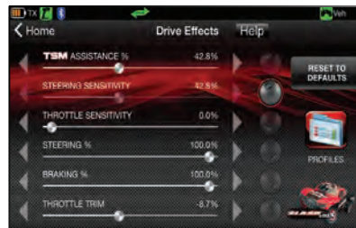
Tap and slide to adjust TSM, Steering Sensitivity, Throttle Trim, Braking Percent, and more!
