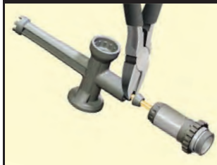
C. Remove/Install Rod End
